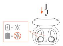
**NOTE** If the charge case has no charge, first charge the case separately, then charge the earbuds.
